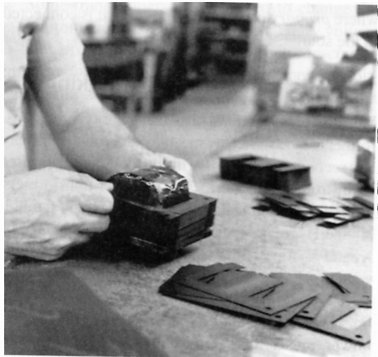
Figure 10.9b Stacking laminations inside a coil.
