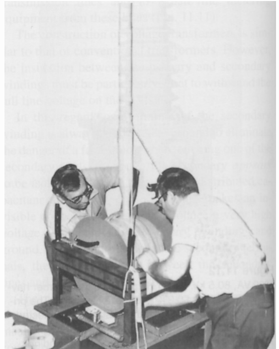
Figure 11.15 Current transformer in the final process of construction. (Courtesy of Ferranti-Packard)
