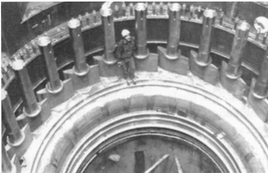
Figure 24.12 Inside the spiral case, a set of adjustable wicket gates control the amount of water flowing into the turbine. (Courtesy of Marine Industrie)
