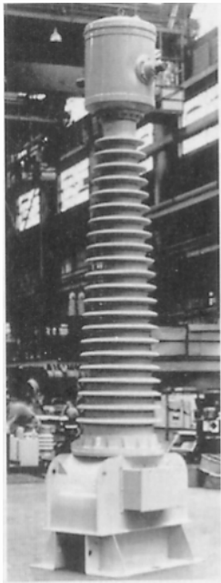
Figure 11.14 500 VA, 100 A/5 A, 60 Hz current transformer, insulated for a 230 kV line and having an accuracy of 0.6%. (Courtesy of Westinghouse)
