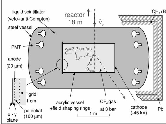
Figure 1. The MUNU detector at the Bugey reactor.
